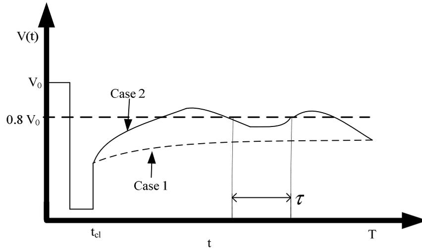
Figure 2.2 Different cases of unacceptable duration of low voltage.
