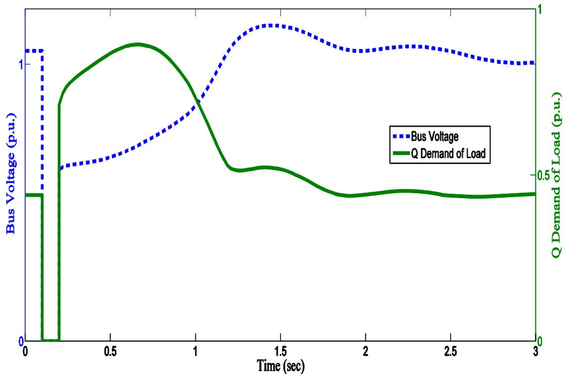
Figure 2.5 Bus voltage and Q demand @bus 119 due to contingency 19-21 w/o SVC.
