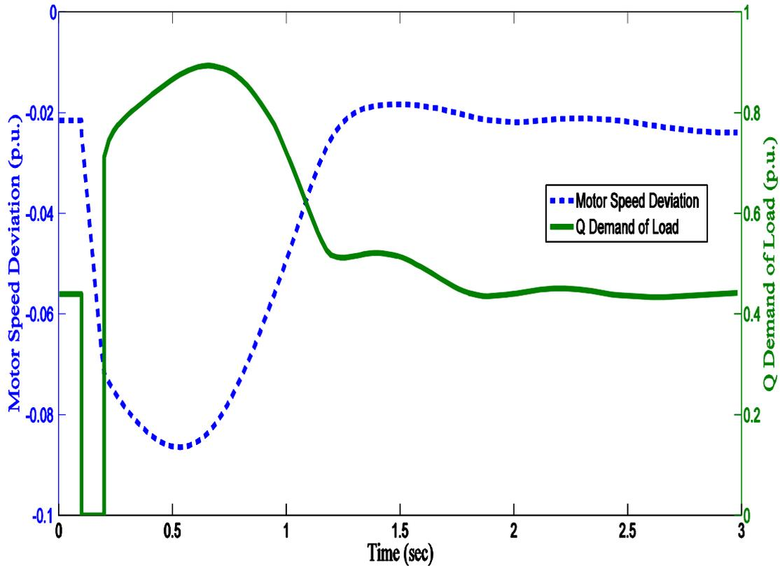
Figure 2.6 Motor speed deviation and Q demand @bus 119 due to contingency 19-21.
