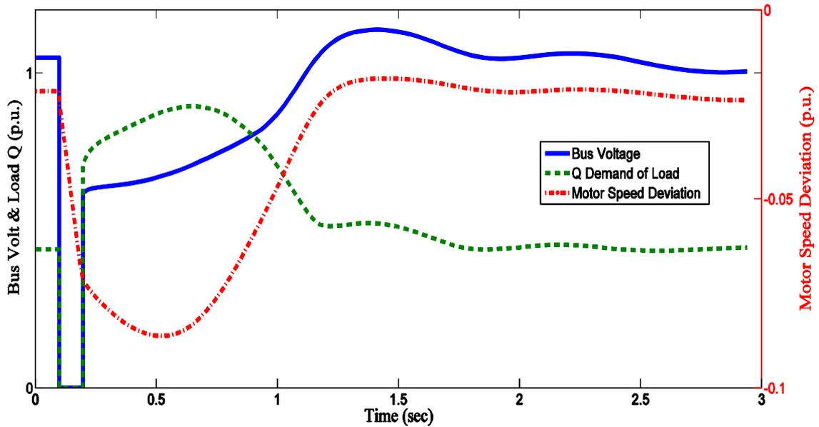
Figure 2.7 Bus voltage, Q and motor speed @bus 119 due to contingency 19-21.
