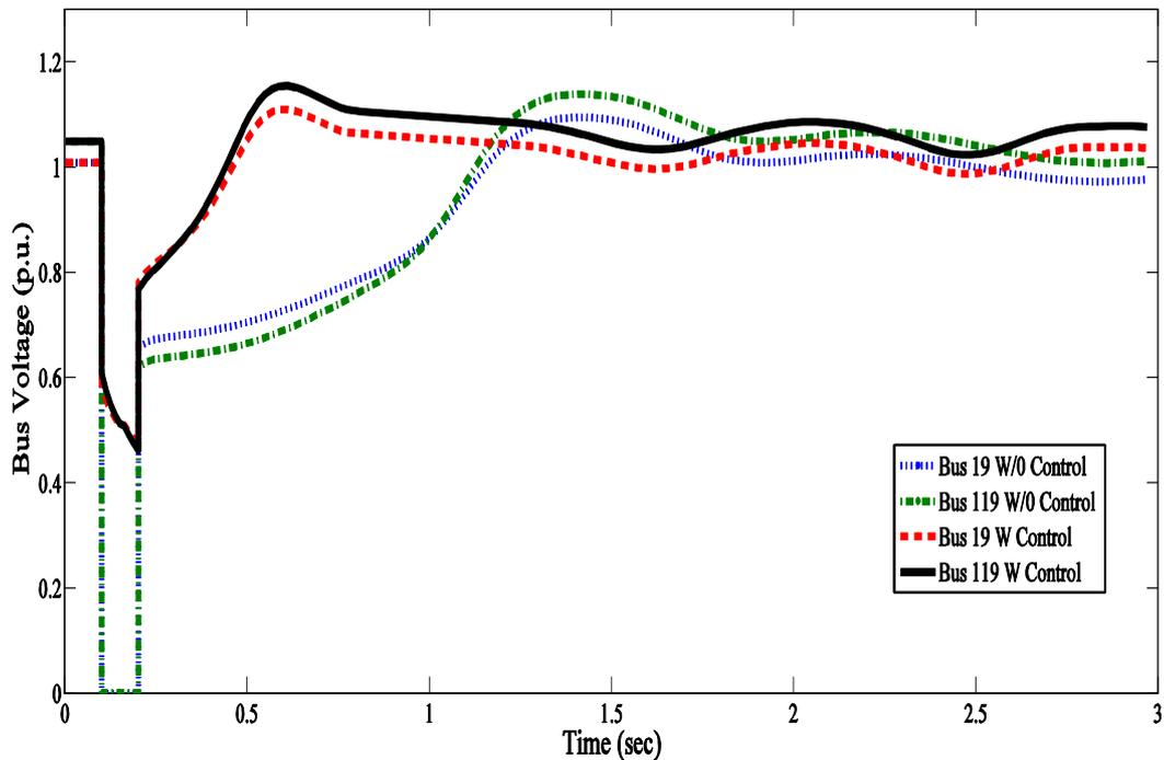
Figure 4.4 Bus voltage response due to line contingency 19-21 with and w/o SVC.
