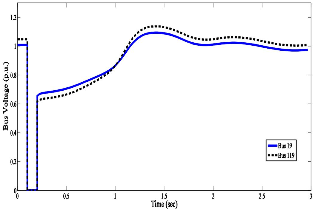
Figure 2.4 Bus voltage response due to contingency 19-21 w/o SVC.
