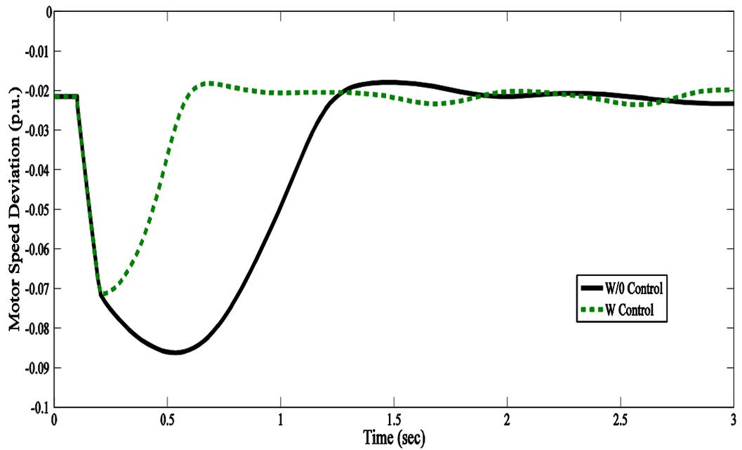
Figure 4.6 Motor speed dev. @bus 119 due to contingency 19-21 with and w/o SVC.
