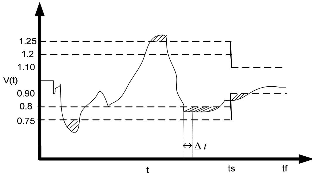
Figure 4.3 Transient voltage dip, and voltage recovery constraint.
