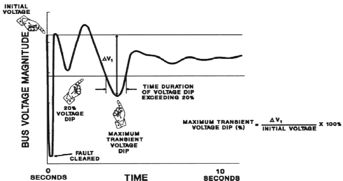
Figure 1.1 Voltage performance parameters for NREC/WECC planning standards.
